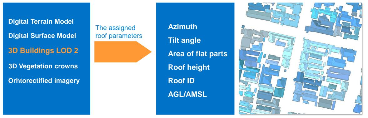
The roof parameters are calculated for each element separately, creating the background for producing solar rooftop maps (solar cadaster)
