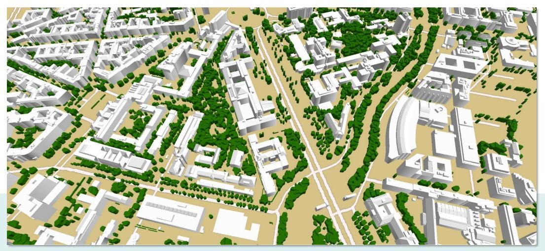
LOD2 3D buildings with sloping roof elements along with 3D vegetation are key initial sources for evaluating solar resource availability and running solar energy simulations
